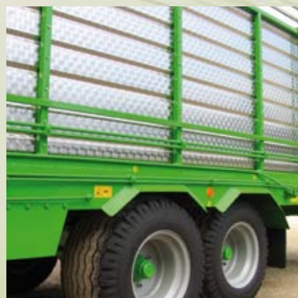
STAINLESS STEEL SIDERAILS STAINLESS STEEL OIL TANK, BED FLOOR AND SUMP ON
