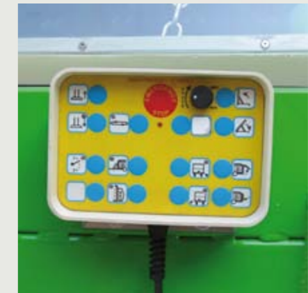
ELECTRONIC BOARD WITH SPEED CONTROL SYSTEM FOR THE UNLOADING CONVEYOR BELT AND EMERGENCY STOP BUTTON
