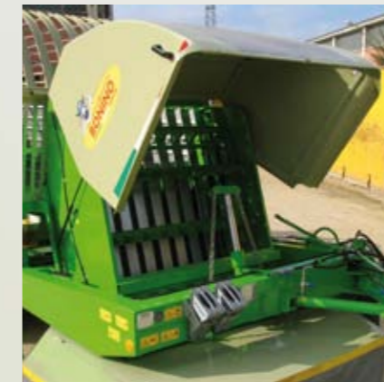
FIBREGLASS BODY WITH WINDOWS TO ACCESS THE GRASS ELEVATOR
