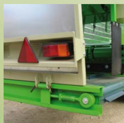
CONVEYOR BELT WITH CONTROL TENSION DEVICE
