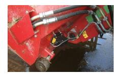
The IRM NIR Analyzer is mounted on the scraper of the front miller and performs a real-time NIR dry matter and nutrient analysis during the loading of each ration ingredient.
