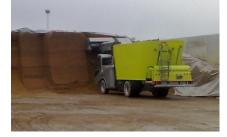
The operator can then add or subtract to the volumes of ration ingredients loaded into the TMR mixer in order to more accurately match the nutritionist's recommendation for each batch of feed.
